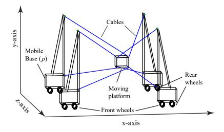
Fig. 1: Concept idea for Mobile Cable-Driven Parallel Robot (MCDPR) with eight cables (m = 8), a six degree-of-freedom moving-platform (n = 6) and four mobile bases (p = 4)
