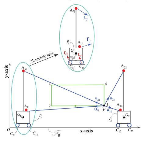
Fig. 2: Point mass Mobile Cable-Driven Parallel Robot with p = 2, n = 2 and m = 4
