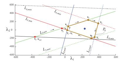
Fig. 3: Feasible Polygon considering only tension limit constraints
