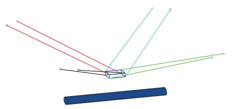
Fig. 7 One configuration of the reconfigurable CAROCA prototype and a cylinder in its working area
