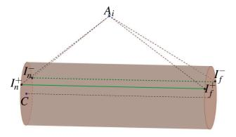
Fig. 4 Boundaries of the interference region between cable  $\mathscr{C}_i$  and the cylindrical part of  $\mathscr{C}$
