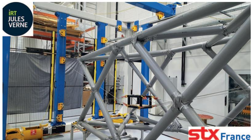
**Fig. 1** CAROCA prototype: a reconfigurable cable-driven parallel robot working in a cluttered environment (Courtesy of IRT Jules Verne and STX France)
