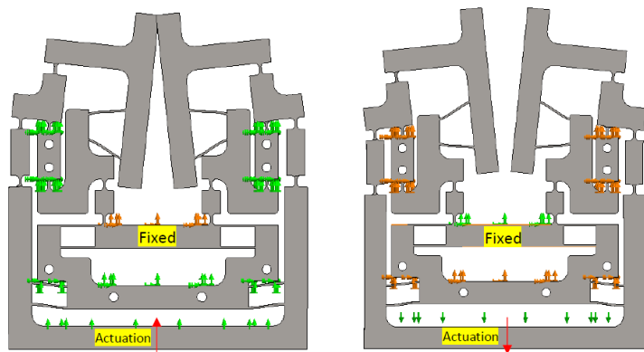
(a) Angular grasping mode 1 : \alpha \neq 0, \beta = 0
