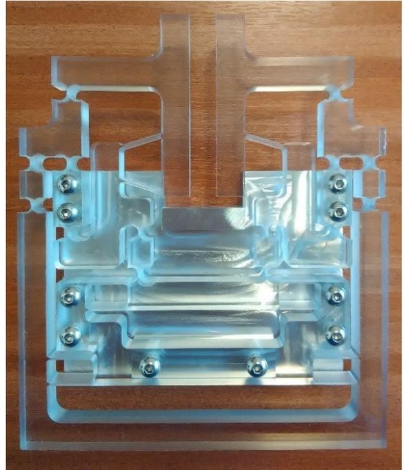
**FIGURE 16: Prototype of the reconfigurable compliant gripper**
