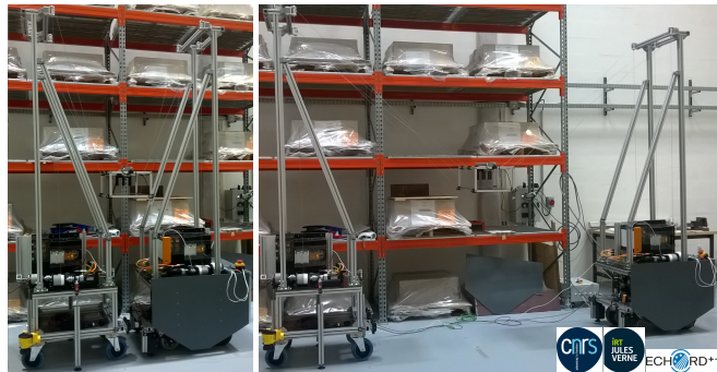
Fig. 1: Fastkit prototype, Undeployed configuration (left) Deployed configuration (right)
