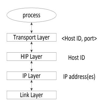
Figure 3. HIP layer within the TCP/IP stack.
