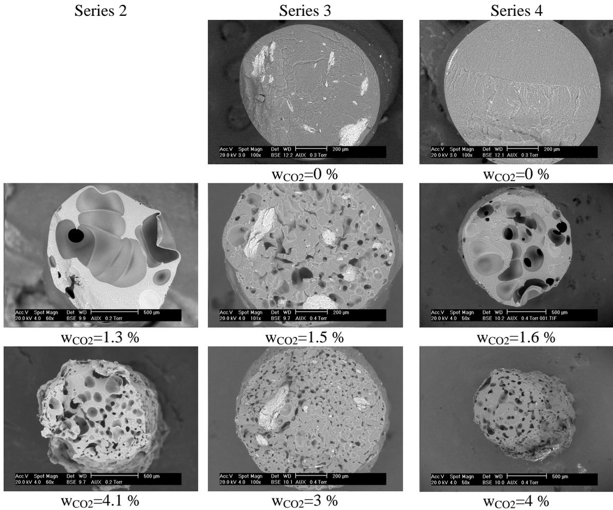
**Figure 9. SEM pictures for series 2 to 4 at different CO<sub>2</sub> mass fraction**
