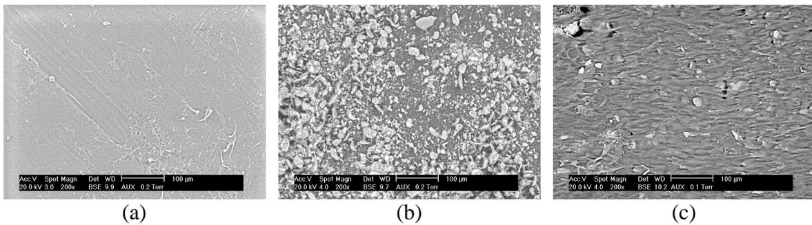
**Figure 3. SEM pictures; (a) PHB-HV; (b) PHB-HV/C30B physical mixture; (c) PHB-HV/C30B extruded mixture**
