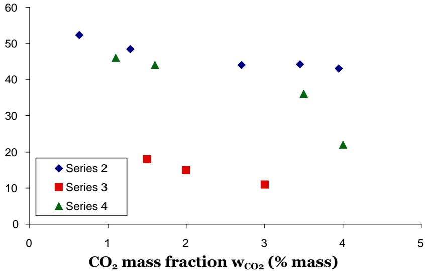
Figure 8. Evolution of the porosity ε with the CO<sub>2</sub> mass fraction
