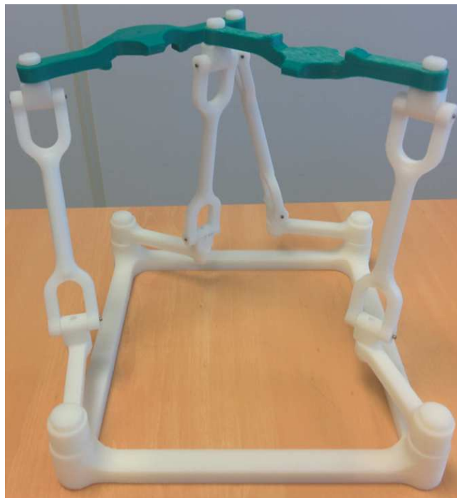
Figure 5: Printed model of 4-RUU PM decomposed into two 2-RUU PM.
