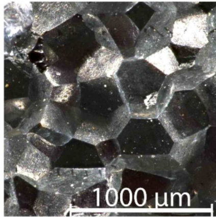
Supplementary Figure 10: Microscope image of the post-mortem fracture surfaces corresponding to the experiments analyzed in Figs. 2 and 3 in the main text. Note the facet-like structure illustrating the intergranular fracture mode and the absence of visible porosity.
