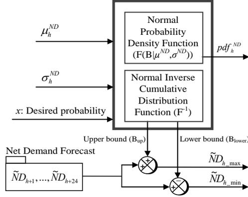
Fig. 5 Net uncertainty calculation at hour  $h$  with a given probability.
