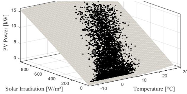
Fig. 2. Irradiance and Temperature vs. Power correlation.
