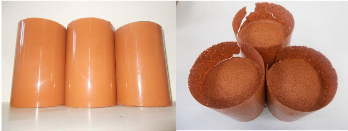
Figure 3. (a) Samples after unmoulding ( HP_1S_{0.008} ); (b) HP_{1.5}S_{0.001} samples with coalescence problems.
