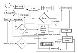
Figure 2: The simple work flow of the mobility management
