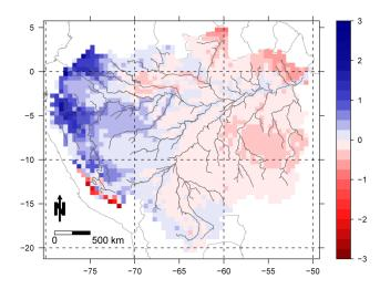
**Fig. 7.** Lengthening (blue) and shortening (red) of duration of inundation in months (mean over 24 model realisations) between future and reference period.
