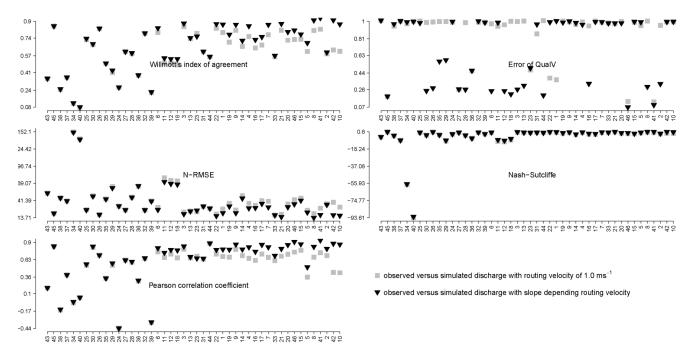
Fig. 4. Comparison of observed and simulated discharge for all 44 observation sites with 5 indices (details in Table 5). Sites are sorted according the observed mean annual discharge [ $m^3 s^{-1}$ ], with the lowest discharge site at the left hand site.
