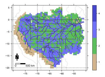
**Fig. 5.** Fraction classes of floodable area per cell. Class 1 representing < 5%, class 2 representing  $\ge 5-10\%$ , class 3 representing  $\ge 10-15\%$ , class 4 representing  $\ge 15-45\%$  of floodable area. For a comparison of simulated floodable area with floodplain area (rectangles R1–R3) see Table 6.
