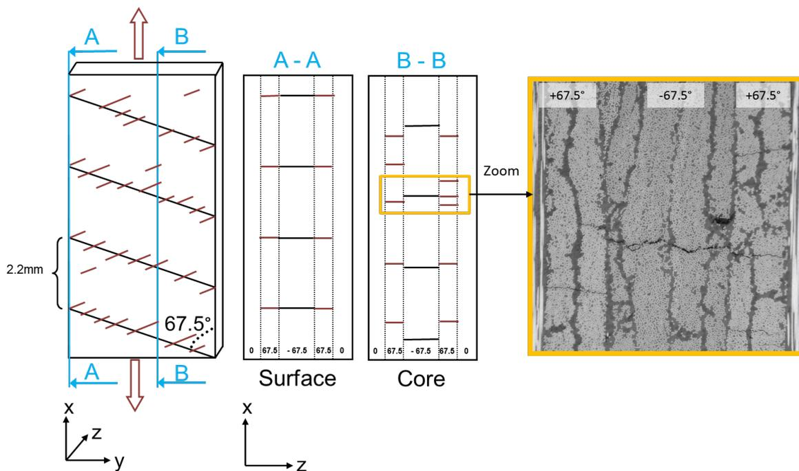
Fig. 9. Crack network in a  $[0/+67.5/-67.5]_s$ : diagram of the network and micrograph of the three damaged plies.
