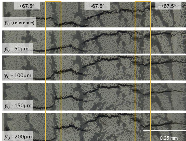
Fig. 10. Intersection between the cracks of three plies in a  $[0/+67.5/-67.5]_s$  for several polishing depth.
