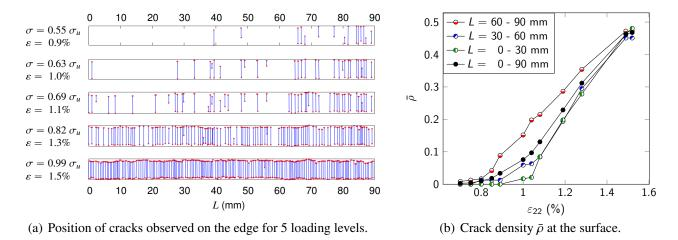
Fig. 7. Damage measurements on a  $[0_2/90_1/0_2]$  specimen, ply thickness  $h_{90} = 0.26$  mm.
