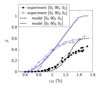
Fig. 8. Measured and predicted crack rates.
