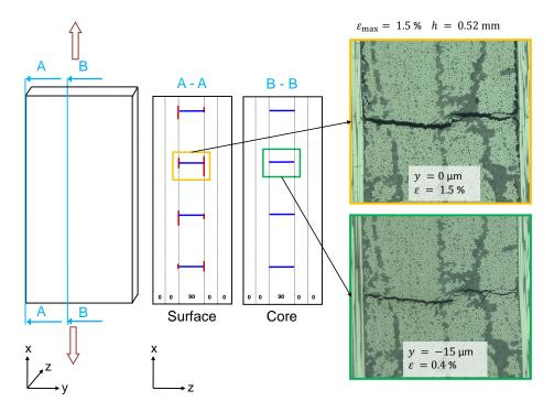
Fig. 4. Cross-section examinations on  $[0_2/90_2/0_2]$ : diagram of the cross-sections and micrographs at the surface  $(y = 0 \mu m)$  and after removing 15 microns  $(y = 15 \mu m)$ .
