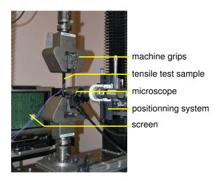
Fig. 3. Damage observation under tensile loading test.
