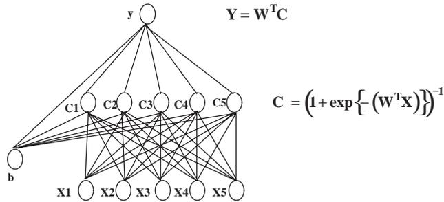
Fig. 1. Scheme of a feed-forward multi-layer perceptron.
