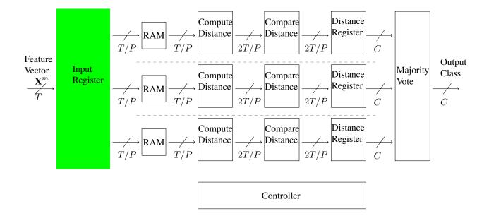
Figure 2. Hardware architecture of ILOC
