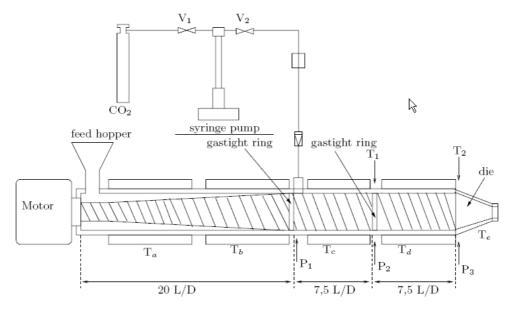
There are three pressure and two temperature sensors:  $P_1$  after the  $CO_2$  injector,  $P_2$  and  $T_1$  before the second gastight ring and  $P_3$  and  $T_2$  by the die. This allows measuring the temperature and the pressure of the polymer inside the extruder. Errors associated to pressure and temperature measurements were about 0.2 MPa and 1°C respectively.
