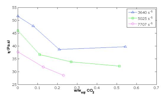
The behaviour in terms of shear rate is not surprising since polymers are often shear thinning. The decrease in viscosity related to  $CO_2$  addition is also consistent with literature observations. This decrease usually follows a power law [13]. However, our measurements suggest a plateau, which is not consistent with such a law. This may be due to the desorption of the  $CO_2$  in the die and the occurrence of a two-phase system that could disturb measurements.
