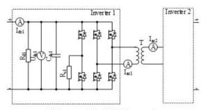
(a) diagram of the DC-DC converter
