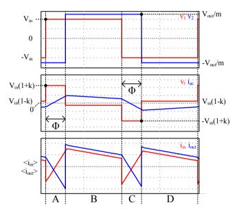
Fig. 2. Thoretical waforms for the phase shifted modulation.
