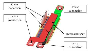
Fig. 3. Internal view of the SiC based power module.
