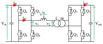
Fig. 1. The Dual Active Bridge topology
