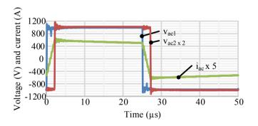
Fig. 11. Waveforms of one DAB converter (V = 1 kV ; k = 1 ;  $P_{dc}$  = 100 kW).
