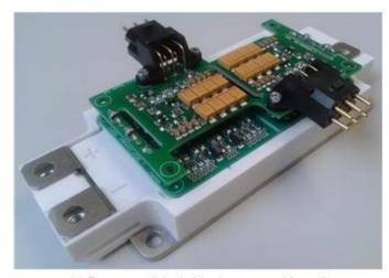
(a) Power module (with close control board)
