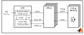
Fig. 9. Architecture of the integration model in Simulink
