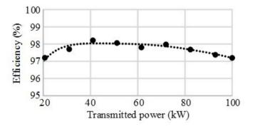
Fig. 12. Efficiency estimation for the standelone (two inverters + two transformers) configuration for the input voltage of 1 kV.
