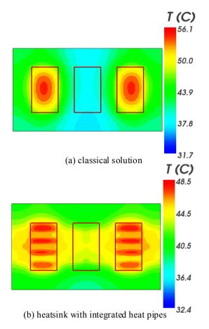
Fig. 4. Thermal simulations of the heatsink for an ambiant temperature of 30 °C and a dissipated power of 1 kW (500 W for each power module). The results were obtained using R-Tools software [10].
