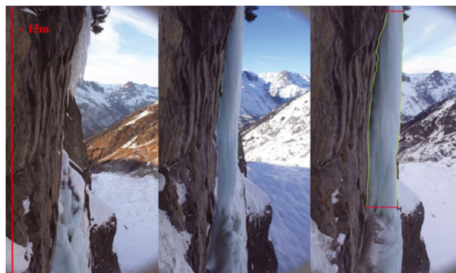
Fig. 6. Evolution of the Nuit Blanche free-standing section, automatically recorded by the camera (sample). From left to right: 28 November 2007, 17 December 2007 and 1 January 2008. The green curve indicates the contour selected for the area measurement. The horizontal borders were kept fixed (red horizontal lines).
