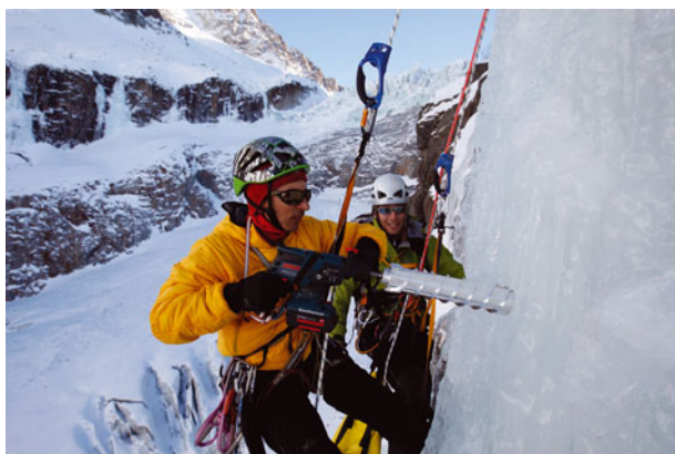
Fig. 5. Coring in the Nuit Blanche free-standing section.
