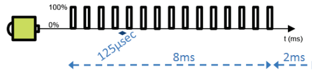
Figure 4: 30-FPS video stream send under AVB SR-A with a 703 bytes Ethernet frame every 125us. 64 frames are sent over 8ms.
