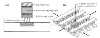
Figure 5. (a) Scheme of typical RRAM memory element: resistive switching layer is sandwiched between top and bottom electrodes to form simple MIM (Metal/Insulator/Metal) structures. (b) Crossbar-type memory architecture in which memory elements are located at the intersections of per-
