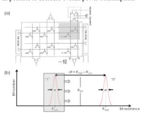
Figure 7. (a) Architecture that enables sensing the resistance state of a programmable conductor random access memory element using complementary resistive elements (dashed square). (b) Bit cell resistance distributions of "0" and "1" resistance states.
