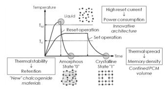
Figure 3. Temperature profiles used for set and reset operations in PCM. Innovations are mandatory to improve data retention, reduce power con-
