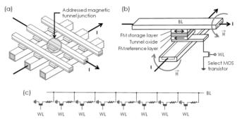
Figure 2. (a) To write MRAM bit, currents are passing through perpendicular metal lines surrounding MTJ. (b) The resultant magnetic fields enable programming a bit in reversing magnetization of upper FM storage layer (select MOS transistor is OFF). To read a bit, a current is passing through the MTJ and its resistance is sensed (select MOS transistor is ON). (c) Schematic diagram of series-parallel architecture for 1T/1MTJ cells.
