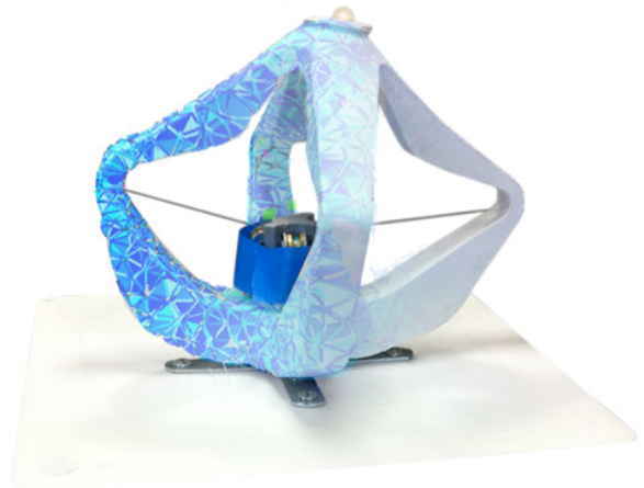
Fig. 11: Deformable parallel manipulator.
