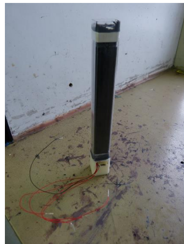
Figure 6. Cassis – Micro-ignition stage & semi-inert pyrotechnical loaf prototype
