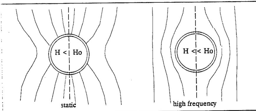
Fig. 3: Flux lines plot (schematic)
