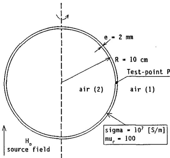
Fig. 2: definition of the test-problem: the hollow ferromagnetic and conducting sphere in a constant field
