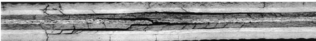
Fig. 13. Micrograph of a section tangent to the hole of a [0_3/\pm 45_2/90]_s specimen at 92% of the rupture load.
