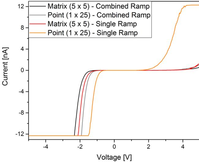
FIG. 3. Comparison of different I-V curve measurement approaches, “matrix” versus “point” and “combined ramp” versus “single ramp”. “Matrix” defines the average curve of the measurements in a  $5 \times 5$  array in contrast to the 25 measurements in a single “point.” For “single ramp,” voltage ramps were applied in one ramp from  $-5$  V to  $5$  V. The “combined ramp” is a combination of two split measurements from  $0$  V to  $\pm 5$  V.
