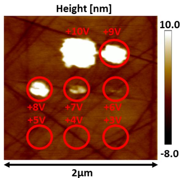
FIG. 1. Tapping mode measurement of a non-irradiated SiC sample after performing different I-V ramps from 0 V to a maximum voltage (i.e., 3 V to 10 V) as indicated in the figure. The red circles help guide the eye to the dedicated spots of the applied ramp (except for the highest voltage).
