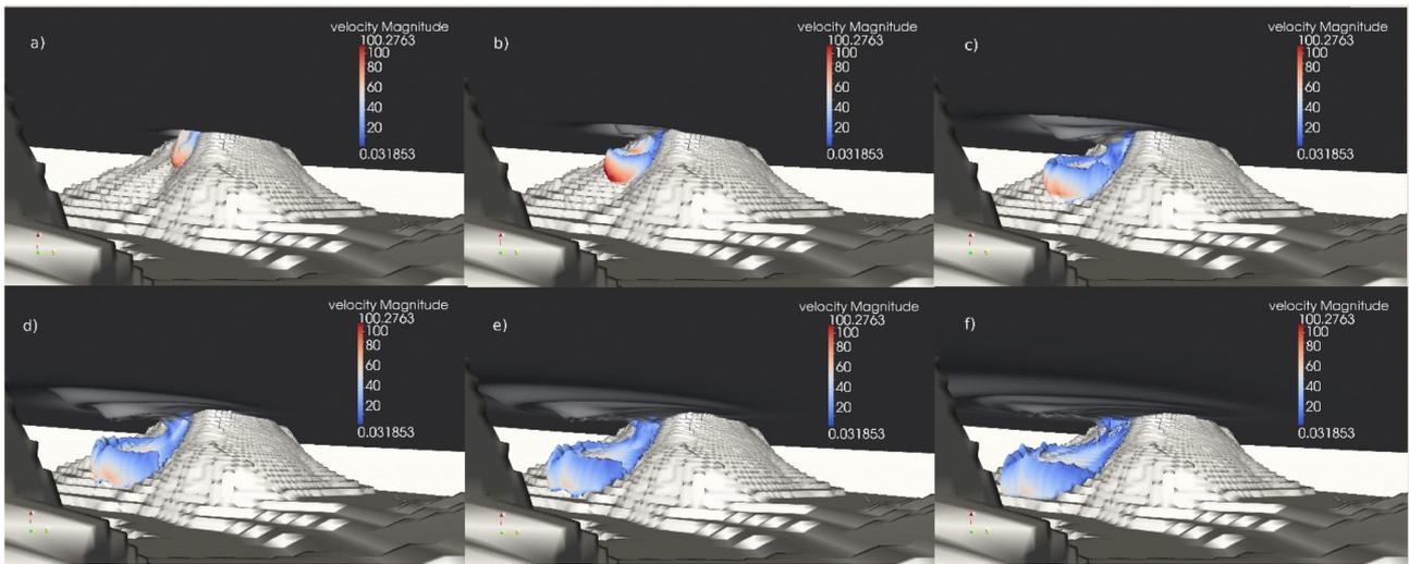
Figure 9 : THETIS 3D computations. Underwater view of water and slide interfaces (volume fractions respectively equal to 0.5 and 0.1) at  $t =$  a) 50 s, b) 100 s, c) 150 s, d) 200 s, e) 250 s, f) 300 s for a slide initial volume of  $80 \text{ km}^3$ . The vertical  $z$  coordinates have been exaggerated by a factor of 5, to allow for a better view of the wave field and slide motion. Slide contour are colored by velocity magnitude.
