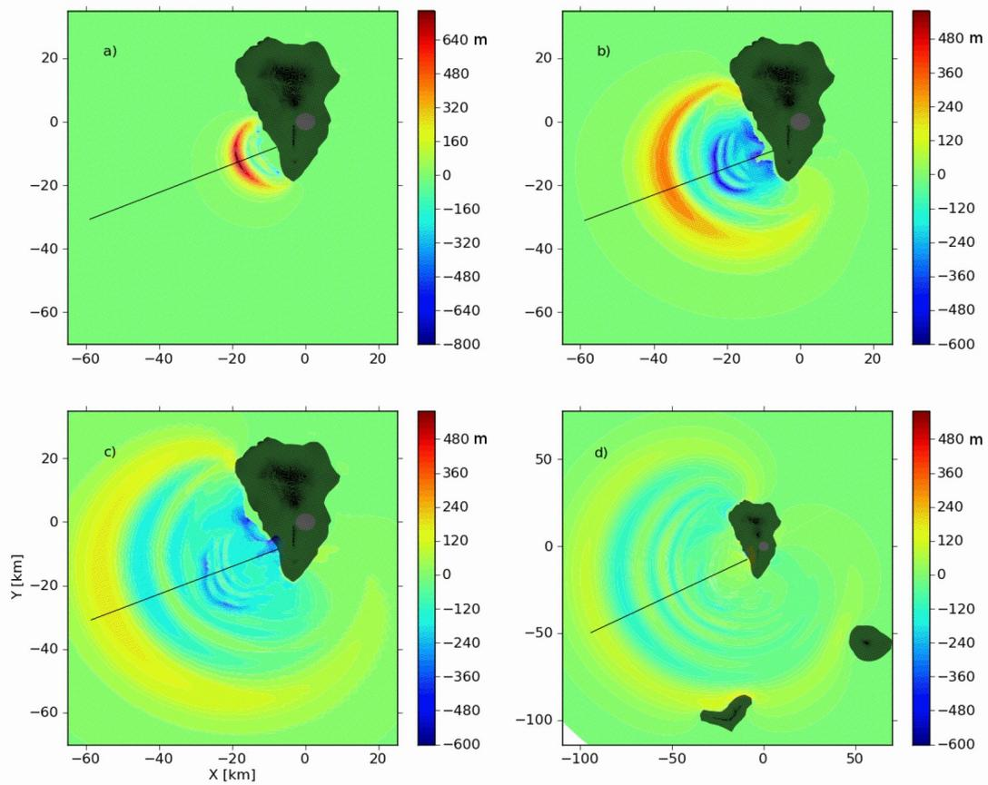
Figure 11 : THETIS 3D computations for  $80 \text{ km}^3$  slide volume. Contours of wave field at  $t =$  a) 101 s, b) 232 s, c) 340 s and d) 558 s.
