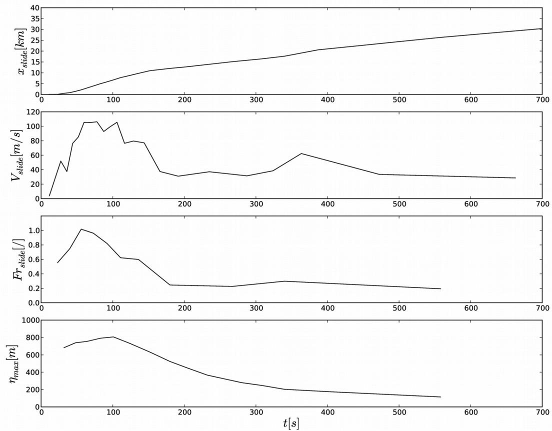
Figure 10 : THETIS 3D computations for  $80 \text{ km}^3$  slide volume. Evolution of slide characteristics with time in a vertical plane  $20^\circ$  anticlockwise with respect to West : a) slide tip distance to shore ; b) slide tip velocity; c) Slide local Froude number ; d) Maximum free surface elevation.
