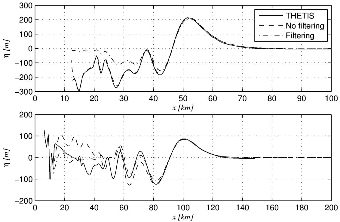
Figure 20 : Transects (see Fig. 19) of surface elevation at  $t = 300$  s (top) and  $t = 550$  s (bottom), as a function of the westward propagation distance. Results show the effects of filtering in FUNWAVE. Note the slight difference in the surface elevation far from La Palma – this is due to a slight artifact of the post-processing of the THETIS results, which is removed before initializing the FUNWAVE model.
