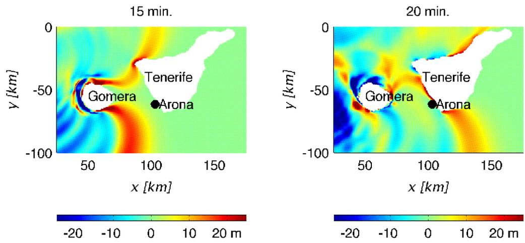
FUNWAVE in a 500 m resolution grid surrounding Tenerife, at 15 min. (left panel) and 20 min. (right panel) after the landslide.
