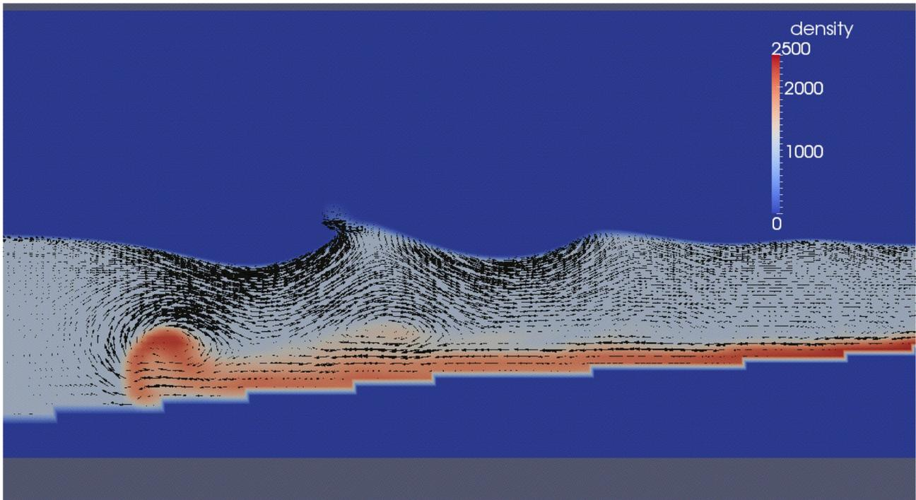
Fig. 6 : Same case as Fig. 4. Detailed velocity field at every other grid around the slide tip at  $t=396$  s, showing the strong current generated in water by the slide displacement and several vortices at the slide/water interface. Maximum velocities in water are on the order of  $100 \text{ ms}^{-1}$ .
