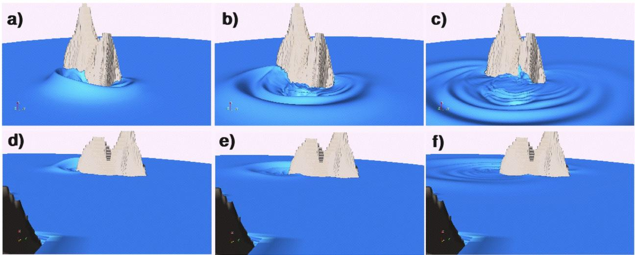
Figure 15 : THETIS 3D computations for  $80 \text{ km}^3$  slide volume. Wave field and run-up on La Palma. South-West view at :  $t =$  a) 192 s, b) 290 s, c) 474 s. East view at  $t =$  d) 192 s, e) 290 s, f) 474 s. Elevation is exaggerated 15 times.
