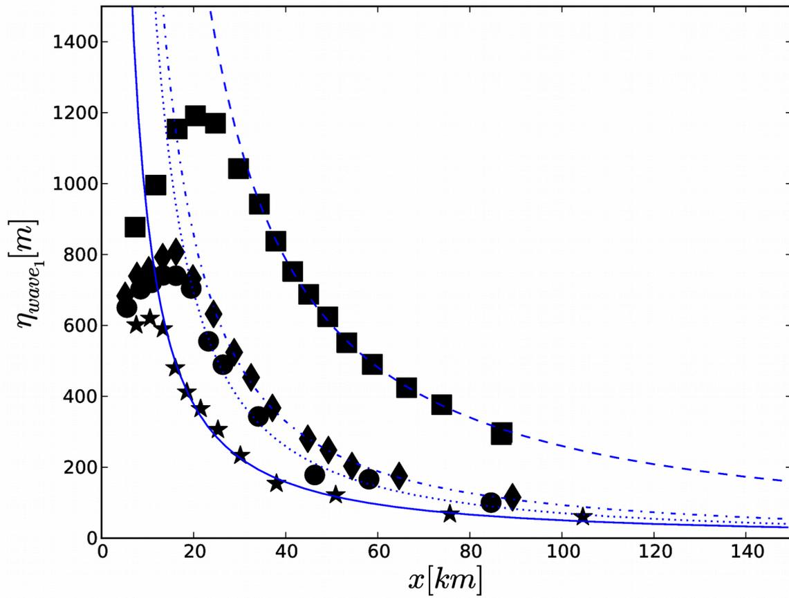
Figure 14 : THETIS computations. Maximum wave elevation decay as a function of distance along transects  $20^\circ$  anticlockwise with respect to West, for the four studied slide volume scenarios (symbols). Curve fitted power laws: solid blue line ( $20 \text{ km}^3$  case),  $r^{-1.25}$ ; dotted blue line ( $40 \text{ km}^3$ ),  $r^{-1.42}$ ; dotted-dashed blue line ( $80 \text{ km}^3$ ),  $r^{-1.38}$ ; dashed blue line ( $450 \text{ km}^3$ ),  $r^{-1.21}$ .
