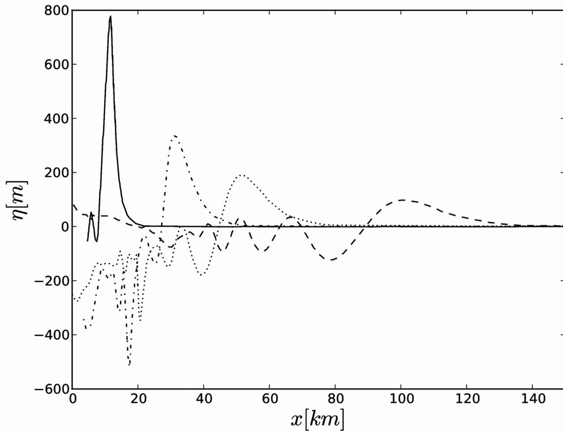
Figure 12 : THETIS 3D computations for  $80 \text{ km}^3$  slide volume. Free surface elevation in a vertical plane  $20^\circ$  anti-clockwise with respect to West, at  $t =$  (solid line) 101 s; (dash-dotted line) 232 s; (dotted line) 340 s; (dashed line) 558 s.
