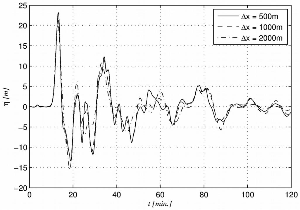
computed surface elevation at the Arona station, for different grid resolutions, from 500 to 2000 m.
