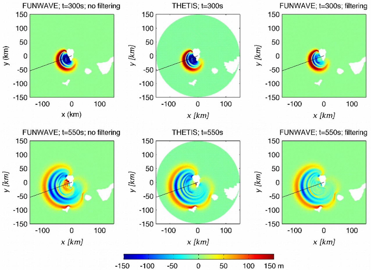
Figure 19 : Test of model coupling for the  $80 \text{ km}^3$  case, when modeling wave propagation from  $t = 300$  to  $550$  s using : (i) FUNWAVE without filtering the initial conditions; (ii) THETIS; and (iii) FUNWAVE with filtering the initial conditions. The main direction of wave propagation,  $20^\circ$  anticlockwise with respect to west, along which transects in Figs. 20, 21, 25, 26 are made, is marked by thin black lines in each subfigure.
