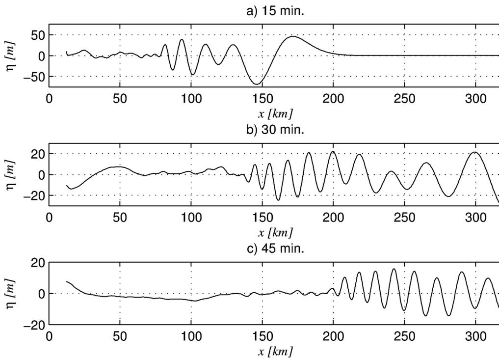
elevation, for the  $80 \text{ km}^3$  slide, at  $t =$  a) 15 min. b) 30 min. c) 45 min., as a function of propagation distance up to the edge of the sponge layer. Results show the long dispersive tail that gradually develops with time.
