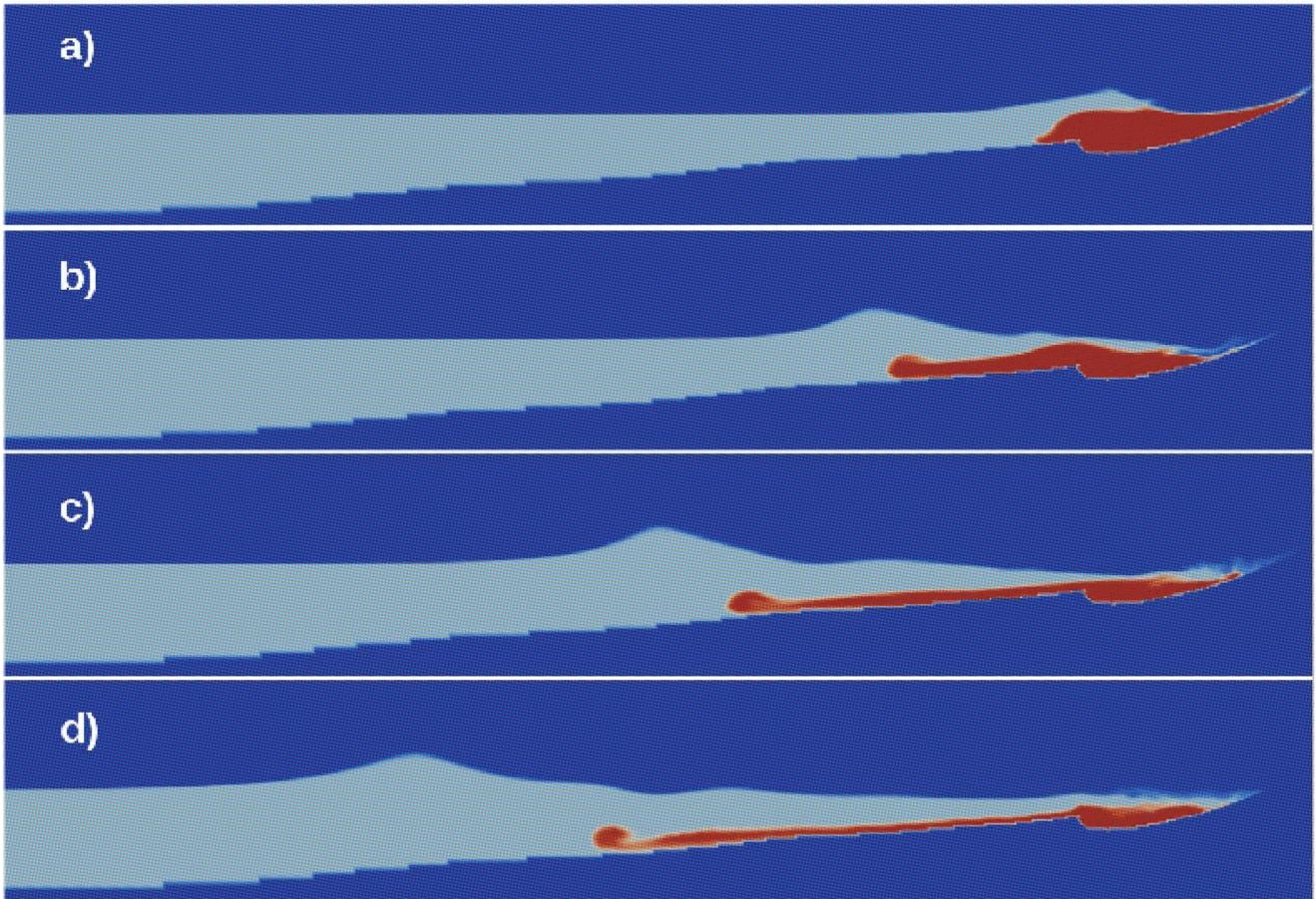
Fig. 4 : THETIS 2D computations with slide initial surface equal to  $8 \text{ km}^2$ . Density contours at  $t =$  a) 50 s, b) 100 s, c) 150 s, d) 200 s.
