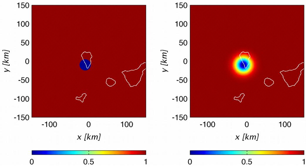
(Gaussian hump with a standard deviation of 15 km, and a center located at (-10 km, -10 km) in the local coordinate system), multiplying wave elevation and horizontal velocity prior to applying the initial conditions of FUNWAVE (right), compared to simple distance criterion (left). Note that if a function like that on the left was used, very sharp edges would exist in the initial condition.
