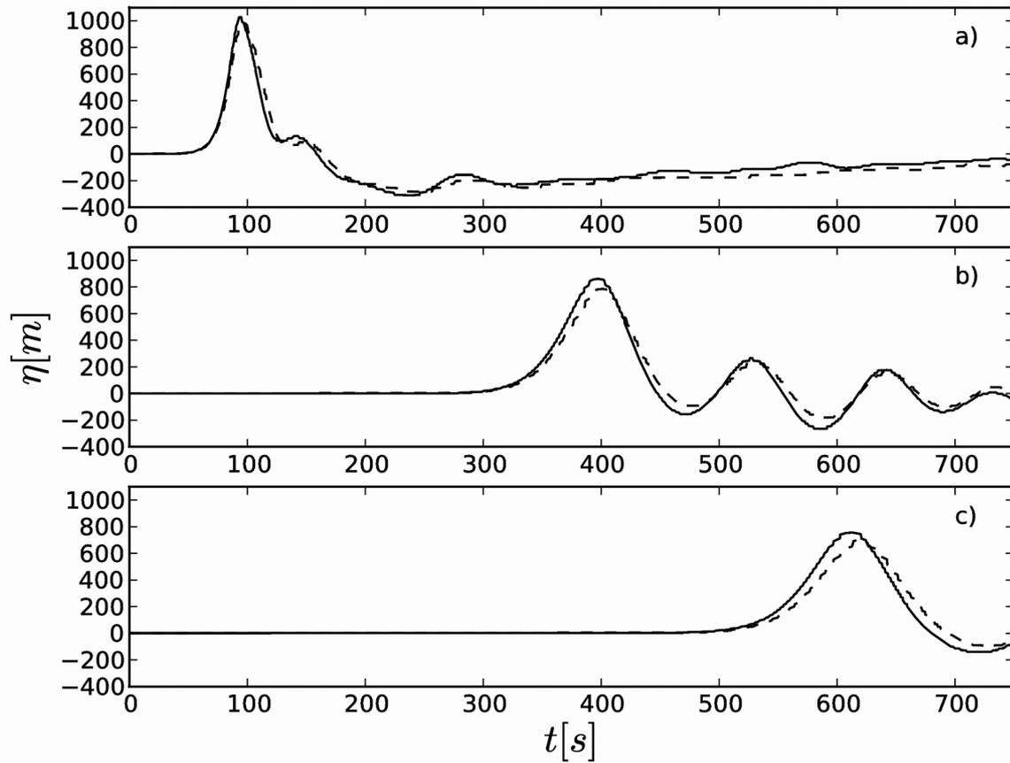
Fig. 3 : Free surface time history (case of Fig. 2) at gage : a) G1 (10 km off-shore), b) G2 (45 km off-shore) and c) G3 (100 km off-shore) for two meshes : mesh 1 (solid line) 1500 x 120 ( $\Delta x=100$  m, irregular in z), mesh 2 (dashed line) 200x80 (irregular in x and z,  $\Delta x_{\min}=100$  m,  $\Delta z_{\min}=10$  m).
