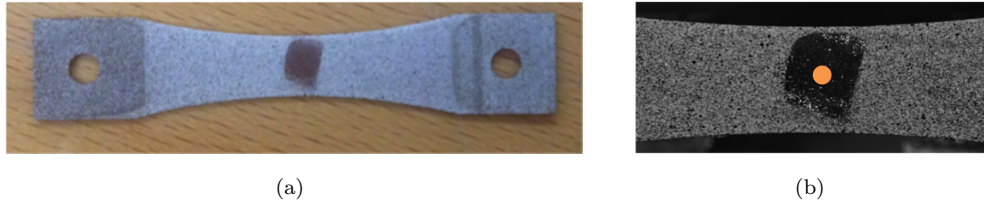
Fig. 9: Coupon for in-situ tests. (a) Dog-bone geometry (ligament width: 6 mm, thickness: 0.5 mm, radius of the hour-glass shape: 65 mm). (b) Speckle pattern used for DIC procedures with an unpainted area to allow for XRD measurements. The area probed by the X-ray beam is depicted in orange.
