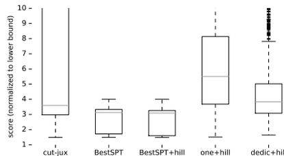
Figure 4: The total cost  $C(P)$  of the solutions returned by various heuristics and by CUTJUXTAPOSE. All algorithms limited to  $10^6$  evaluations. The cost normalized to the lower bound. All instances.
