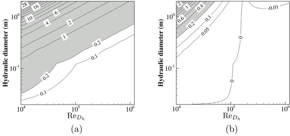
Figure 7: Contour plots of the  $\tilde{\mathcal{I}}$  (a) and  $\tilde{\mathcal{J}}$  (b) indicators as functions of the practical Reynolds number  $Re_{D_h}$  and the channel hydraulic diameter  $D_h$ . The pressure is set to 1 atm and the walls emissivity to 0.8.
