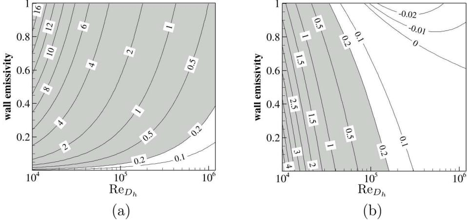
Figure 5: Contour plots of the  $\tilde{\mathcal{I}}$  (a) and  $\tilde{\mathcal{J}}$  (b) indicators as functions of the Reynolds number  $\text{Re}_{D_h}$  and the walls emissivity. The pressure is set to 40 atm and the channel hydraulic diameter  $D_h$  to 0.4 m.
