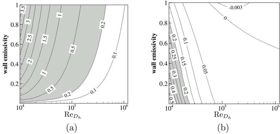
Figure 8: Contour plots of the  $\tilde{\mathcal{I}}$  (a) and  $\tilde{\mathcal{J}}$  (b) indicators as functions of the Reynolds number  $Re_{D_h}$  and the walls emissivity. The pressure is set to 1 atm and the channel hydraulic diameter  $D_h$  to 0.4 m.
