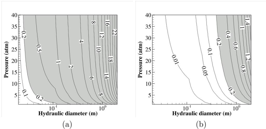
Figure 12: Contour plots of the  $\tilde{\mathcal{I}}$  (a) and  $\tilde{\mathcal{J}}$  (b) indicators as functions of the channel hydraulic diameter  $D_h$  and pressure. The walls emissivity is 0.8 and  $\text{Re}_{D_h} = 48,000$ .
