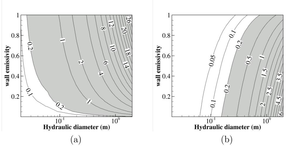
Figure 6: Contour plots of the  $\tilde{\mathcal{I}}$  (a) and  $\tilde{\mathcal{J}}$  (b) indicators as function of the walls emissivity and the channel hydraulic diameter  $D_h$ . The pressure is set to 40 atm and  $\text{Re}_{D_h}=48,000$ .
