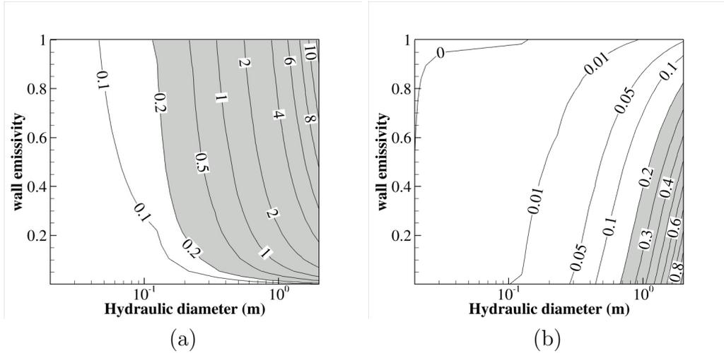
Figure 9: Contour plots of the  $\tilde{\mathcal{I}}$  (a) and  $\tilde{\mathcal{J}}$  (b) indicators as functions of the walls emissivity and the channel hydraulic diameter  $D_h$ . The pressure is set to 1 atm and  $\text{Re}_{D_h} = 48,000$ .
