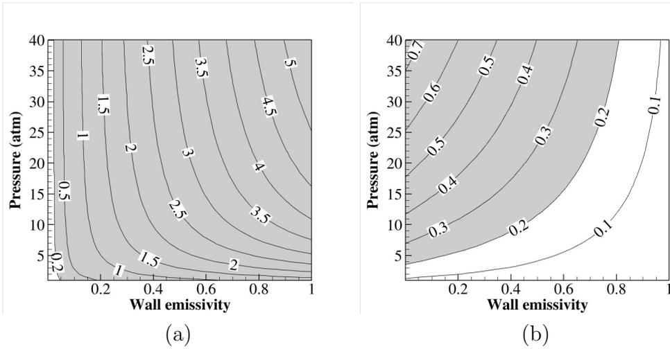
Figure 11: Contour plots of the  $\tilde{I}$  (a) and  $\tilde{J}$  (b) indicators as functions of the walls emissivity and pressure. The channel hydraulic diameter is set to 0.4 m and  $Re_{D_h} = 48,000$ .
