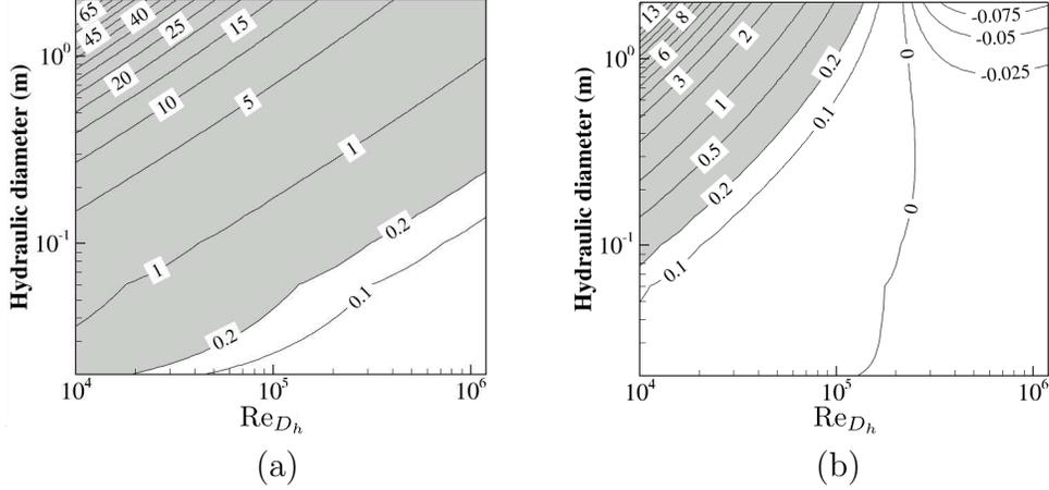
Figure 4: Contour plots of the  $\tilde{\mathcal{I}}$  (a) and  $\tilde{\mathcal{J}}$  (b) indicators as functions of the Reynolds number  $\text{Re}_{D_h}$  and the channel hydraulic diameter  $D_h$ . The pressure is set to 40 atm and the walls emissivity to 0.8.
