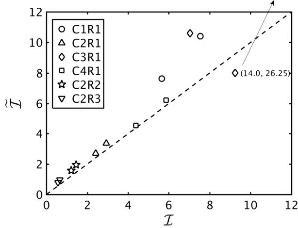
Figure 1: Comparison of indicators quantifying the wall radiative flux: the  $\mathcal{I}$  indicator given by Eq. (2) based on coupled results and the approximating indicator  $\tilde{\mathcal{I}}$  indicator given by Eq. (3). Symbols correspond to results (for both cold and hot sides) of coupled direct numerical simulations in different channel flow conditions denoted by C1R1, C2R1, C3R1, C4R1, C2R2 and C2R3 (see Ref. [8]). The dashed line denotes the identity line.
