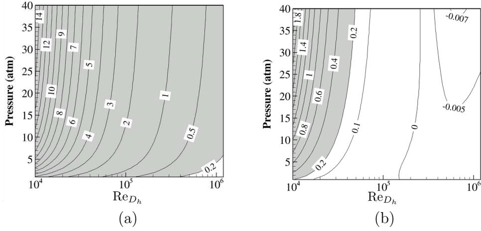
Figure 10: Contour plots of the  $\tilde{I}$  (a) and  $\tilde{J}$  (b) indicators as functions of the Reynolds number  $Re_{D_h}$  and pressure. The channel hydraulic diameter  $D_h$  is set to 0.4 m and the walls emissivity to 0.8.
