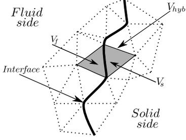
Figure 1: Fluid and solid domains used for a coupled simulation. Dashed triangles represent the cells (actual mesh cells for volume-centred formalism or dual mesh cells for vertex-centred formalism). Both grey triangles denote the fluid and solid cells of volume  $V_f$  and  $V_s$  respectively, which define the hybrid cell of volume  $V_{hyb}$  around the interface.
