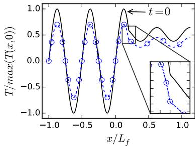
Figure 5: Spatial profiles of the temperature fluctuations scaled by the initial maximal temperature. Black plain line: Temperature at  $t = 0$ . Blue dashed line: Numerically computed temperature profile at  $t = 25$  ms. Blue circles: Analytic manufactured solution at  $t = 25$  ms.
