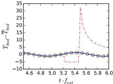
Figure 14: Temporal evolution of the difference of the boundary temperature  $T_{bnd}$  with its mean value,  $\bar{T}_{bnd}$  for the reference solution (circles) and the  $I$  (red dashed-dotted line),  $PI$  (blue dashed line) and  $PID$  (black plain line) controllers. Case conditions:  $\eta = 5\%$  and  $f_{ext} = 5$  Hz.
