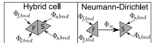
Figure 3: Energy budget in the hybrid cell approach (left) and in the Neumann-Dirichlet method (right). The fluid cell is denoted by F, respectively S for the solid cell.  $\Phi_w$  is the flux sent by the flow solver to the solid solver in the Neumann-Dirichlet method.
