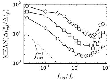
Figure 18: The mean coupling time step scaled by the fluid time step computed by the PID controller as a function of the frequency  $f_{ext}$  for different values of the prescribed tolerance  $\eta$ : 0.05% (line and circles), 0.5% (line and squares) and 5% (line and diamonds). The frequency is scaled by the fluid domain cut-off frequency  $f_c = 25a_f / (\pi L_f^2) = 200$  Hz.
