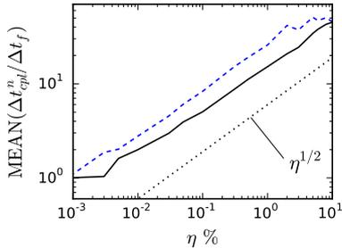
Figure 16: The mean coupling time step scaled by the fluid time step as a function of the prescribed tolerance  $\eta$  for the PI (blue dashed line) and PID (black plain line) controllers. The dotted line indicates a  $\eta^{1/2}$ -law for comparison. Case condition:  $f_{ext} = 100$  Hz.
