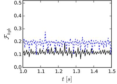
Figure 13: Temporal evolution of the hybrid Fourier number for the simulation controlled by a PID controller for two different tolerances. Black plain line:  $\eta = 1\%$ . Blue dashed line:  $\eta = 3\%$ . Case conditions:  $f_{ext} = 100$  Hz.
