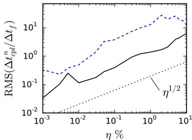
Figure 17: The root-mean-square (RMS) of the coupling time step scaled by the fluid time step as a function of the prescribed tolerance  $\eta$  for the PI (blue dashed line) and PID (black plain line) controllers. The dotted line indicates a  $\eta^{1/2}$ -law for comparison. Case condition:  $f_{ext} = 100$  Hz.
