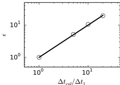
Figure 6: Scaled numerical error of the hybrid-cell computed interface temperature ( $\epsilon$ ) as a function of the coupling step size used. Black circles: Computed error values. Black plain line: Theoretical first order evolution.
