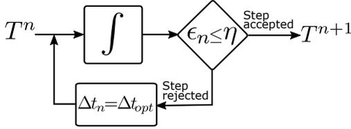
Figure 9: Generic control loop to advance the boundary temperature  $T^n$  to its value  $T^{n+1}$  with a numerical integration error  $\epsilon_n$  below a given tolerance  $\eta$  by adapting the integration time step  $\Delta t_n$ .
