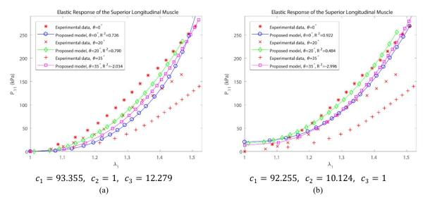
Figure A1. Best fitted curves to the elastic response of the SLM tissue when  $c_2$  was ignored (a) and when  $c_3$  was ignored (b).
