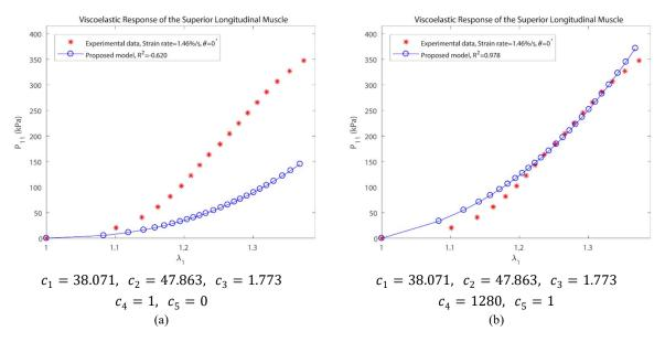
Figure A3. Best fitted curves to the rate dependent response of the SLM tissue when  $c_4$  was ignored (a) and when  $c_5$  was ignored (b).
