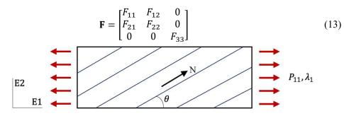
Figure 2. A transversely isotropic sample under uniaxial tension. Fibers are supposed to be fully laid in the E1E2 plane.
