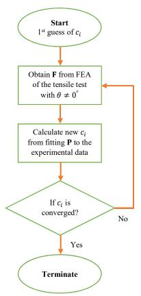
Figure 5. Flowchart of material parameters estimation procedure of a transversely isotropic material from uniaxial tensile tests.
