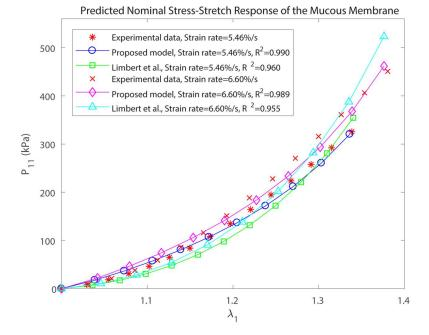
Figure 4. Comparison of the accuracy of prediction of the rate dependent response of the mucous tissue between the proposed model and Limbert's one.
