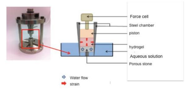
Figure 1: Experimental device develop to characterize swelling of hydrogel in aqueous solutions (Halle mécatronique, LMGC, Montpellier, France).
