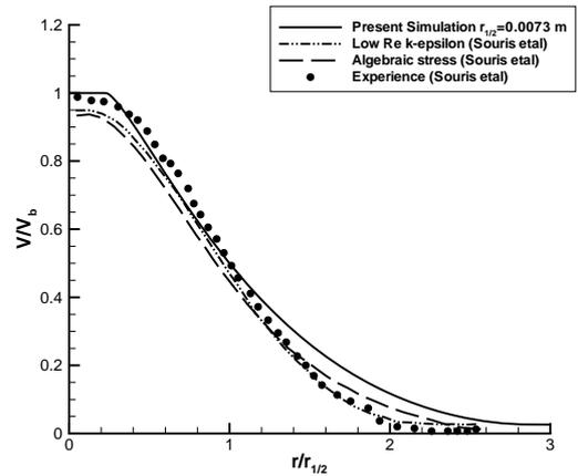
Figure 1: Non-dimensional free-jet velocity profiles for a distance of  $H_p/D_n = 4$  away from the impact surface.  $r_{1/2}$  is the radial distance where  $V = V_b/2$  and  $V_b$  is the fluid velocity at the center line of the jet
