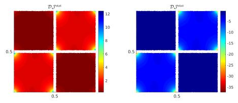
Fig. 4. Distribution of quasi-static sensitivity  $\mathcal{DJ}^{\text{stat}}(z)$  over the unit cell assuming  $\Delta\mu=1$  (left) and  $\Delta\mu=-1$  (right). The near-interface points are omitted from the plot.
