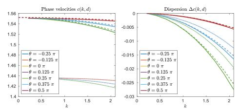
FIG. 3. Left: phase velocity  $c(k, \mathbf{d})$  for the designed chessboard material (homogenized model—dashed, numerical values—solid), and manufactured chessboard material (numerical values—dotted). Right: anisotropic dispersion shown in terms of  $\Delta c(k, \mathbf{d}) = c(k, \mathbf{d}) - c(k_{\min}, \mathbf{d})$ . Note that the results for directions  $\theta = \{0, \pi/2\}$  coincide, as do those for directions  $\theta = \{-\pi/4, \pi/4\}$  and  $\theta = \{-\pi/8, \pi/8, 3\pi/8\}$ .
