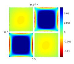
FIG. 5. Distribution of dynamic sensitivity  $\mathcal{DJ}^{dyn}(z)$  over the unit cell assuming  $\Delta\mu=-1$ . The near-interface points are omitted from the plot, and a threshold is applied to the most positive TS values (as only their sign is of interest) so that the color scale is symmetric around 0.
