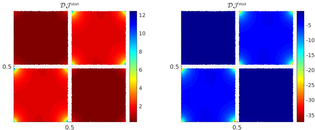
FIGURE 4. Distribution of quasistatic sensitivity  $\mathcal{D}\mathcal{J}^{\text{stat}}(\mathbf{z})$  over the unit cell assuming  $\Delta\mu = 1$  (left) and  $\Delta\mu = -1$  (right). The near-interface points are omitted from the plot.
