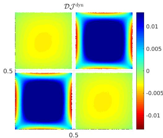
FIGURE 5. Distribution of dynamic sensitivity  $\mathcal{D}\mathcal{J}^{\text{dyn}}(\mathbf{z})$  over the unit cell assuming  $\Delta\mu = -1$ . The near-interface points are omitted from the plot, and a threshold is applied to the most positive TS values (as only their sign is of interest) so that the color scale is symmetric around 0.
