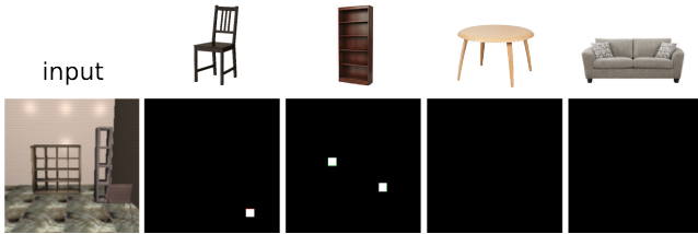
Figure 2: A scene map describes the scene on a per-class basis from a top-down view corresponding to an input RGB image. A white square indicates the presence of an instance of that particular class at that location. Here we show the groundtruth scene map, while our result can be seen in Figure 7, bottom row.
