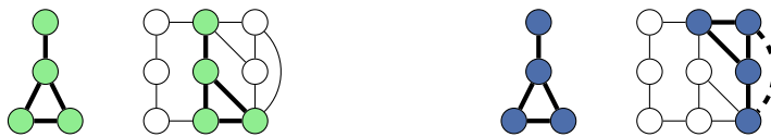
Figure 1: On the left, an induced subgraph isomorphism. On the right, a non-induced subgraph isomorphism: the extra dashed edge is not present in the pattern graph.
