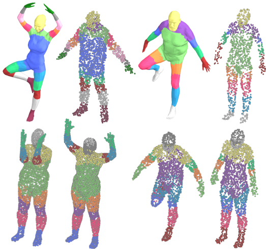
Figure 5: Region-based correspondence between triangular meshes and point clouds (top row), and between point clouds (bottom). The shapes vary in pose, body type, sampling density, and sampling noise.
