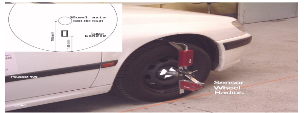
Fig. 5. Sensor for wheel radius measurement
