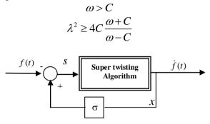
Fig. 2. Structure of the differentiator
