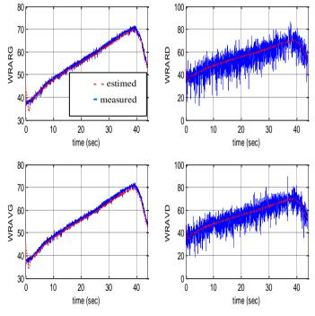
Figure 4. The four wheel rotational velocities
