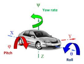
Figure 1: The different movements of the vehicle
