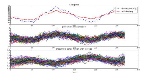
Figure 3: One simulation of spot price (upper graph) without battery in the system (straight line) and with batteries (dashed line), prosumers' original consumption  $Q^i$  (middle graph), and prosumers' net consumption  $Q^i - \alpha^i$  (lower graph) for every prosumers.
