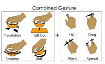
Figure 2. TDome allows performing combined gestures, i.e. a physical manipulation followed by a touch gesture
