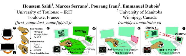
Figure 1. TDome combines a small (a) or large (b) touchscreen with a dome-like mouse [23]. TDome supports performing combined gestures (c), i.e. a 6 DOF physical manipulation followed by a touch input. TDome facilitates several common tasks in MDEs, such as d) display registration using its embedded camera, e) device selection and f) cross-display data transfer.
