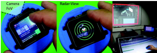
Figure 4: TDome's on-board camera detects displays (left) and creates a radar-view of the spatial layout (center). Then the user can select a display by Rolling + Tapping towards it (right).
