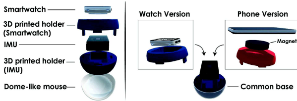
Figure 3. Arrangement of TDome elements for the Small version (left). Both TDome versions are rapidly interchangeable (right).
