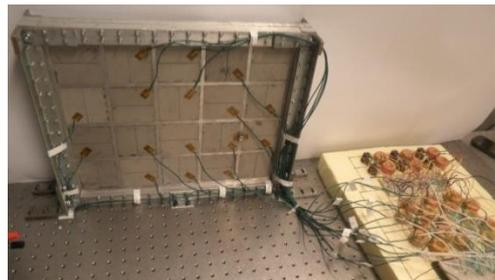
FIGURE 3. PLATE COUPLED TO ITS ANALOGOUS NETWORK
