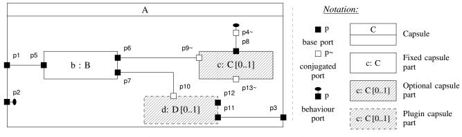
Fig. 1: A UML-RT Structure (Capsule) Diagram
