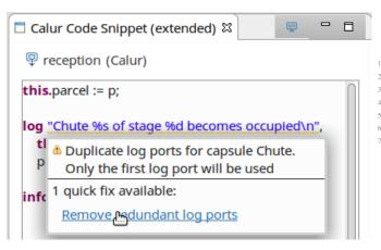
Fig. 9: Warning Message for Duplicated Log Ports
