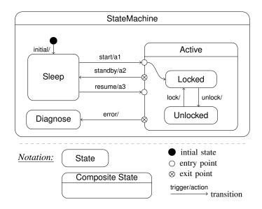
Fig. 2: A UML-RT State Machine Diagram
