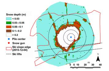
**Figure 3.** The snow depth raster for 23 November 2015 production session along with the positions of the snowgun, the center of the MM snow pile and the concentric circles of radius R = 5, 10, 20 and 30 m. The edge of the ski slope on 4 December 2015 is also shown.
