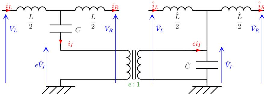
Figure 7: Coupling of two electrical networks
